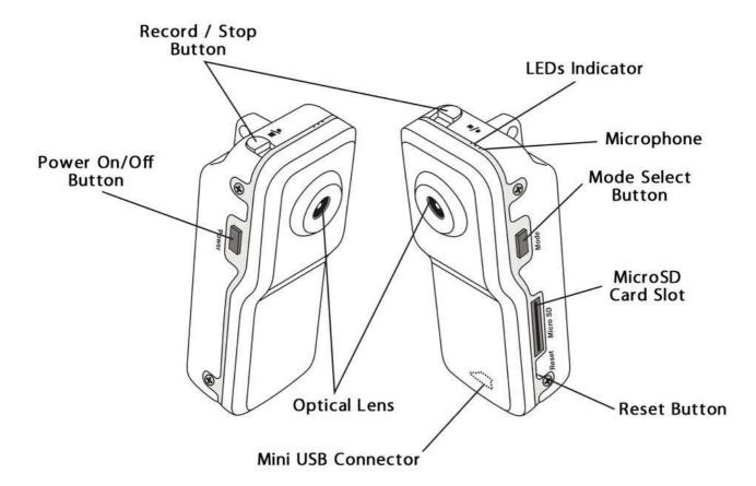
**Lens:** The business-end of the camera, used to focus light on to the image sensor. For best result, ensure the lens is clean and free from debris.
